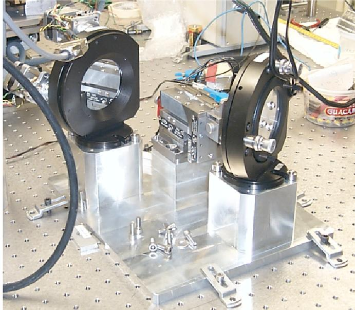
**Figure 2.** Input stage used to optimize the injection. The plan mirror (left) collects the beam from the telescope and sends it the off-axis parabola (right, behind the mount) in order to focus on the single-mode fiber. The plan mirror mount can be tilted in order to change the star position on the focal plan and thus optimize the injection in the fiber. This process, fully automated, increases the efficiency of the remote mode.
