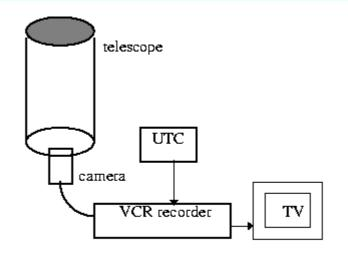
Fig. 1 - The connection telescope/camera/VCR.
